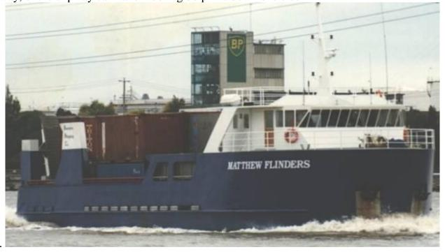
The Mathew Flinders 35 metre commercial Stern Loading Vessel suitable for Isles of Scilly route. Capacity up to 300 tonnes of general cargo in industry standard containers and stillages, and 24 Passengers
