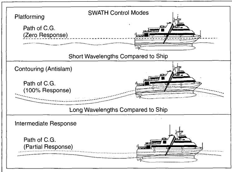
Fig. 4. Modes of automatic ride control (courtesy of Swath International Limited).
