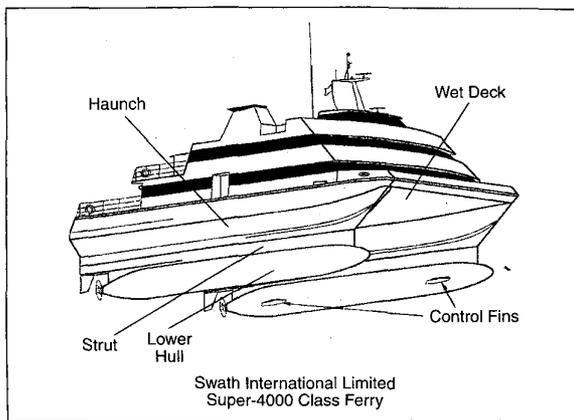
**Fig. 2.** Typical design geometry for SWATH (courtesy of Swath International Limited).
