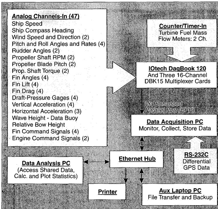
Fig. 5. Block diagram of the measurement path (courtesy of Swath International Limited).
